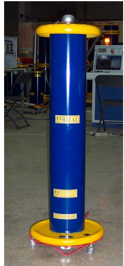
240kV Impulse Voltage Divider
